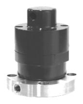
The Rotorseals type Dp-2G and Dp-3G allow for the transfer of media thru two separate shaft passages that are located on the same shaft end. Each passage can be used for a different medium, operating at continuous or intermittently with high speeds, in one or various directions. Both the inlet and outlet ports have American National Pipe Threads.
