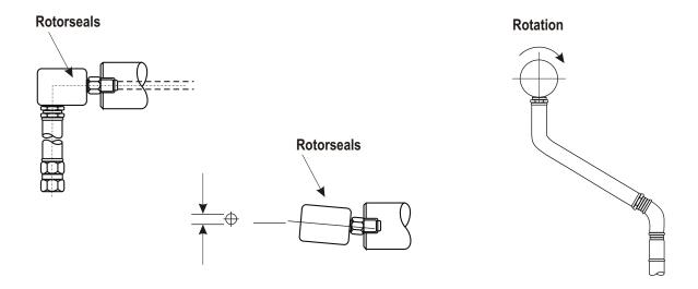
It is important to make the flexible connection between pipe and rotorseal prior to mounting the rotorseal to the rotating body. These well help avoid seal and bearing damage. The connection to the supply line by the union should be done last.
