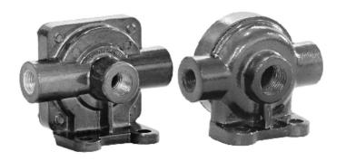
The quick release valve W type reduces the required time for the air relief under pressure of a cylinder or pneumatic device, exhausting it directly into the atmosphere. This kind of design is connected to the air pipe medium, generally located before the Rotorseal.
