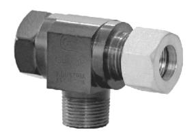
The quick release valve FK type provides for an immediate positive release of the compressed air. They are designed with a piston of low weight that allows for a fast action that assures a long operating life of the valve.
