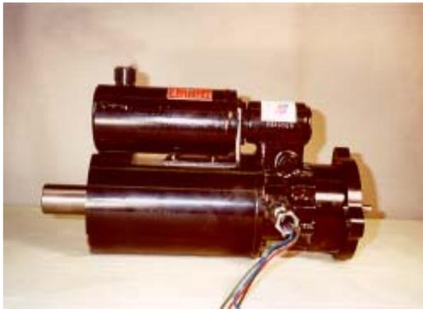
The Electric Starter Drive is in a self-contained package and is used to link an electric motor to the engine. Positively engaged and pre-engaged clutches are applied. Solenoid and pneumatic-actuated designs are used.
