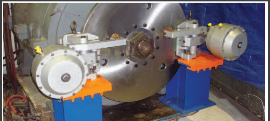
Hoist Motor Brakes Coremo E4N-BP on SMI Floating Bracket
